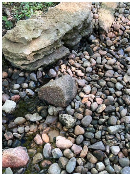
Photos taken from 6-24-2020 site visit. Left – area to add 12" boulder material to slow velocity; Middle – size reference of existing material onsite of large boulder measuring 3-4' long, medium 8-12", and small 3" pebbles; Right – 12-18" boulder
